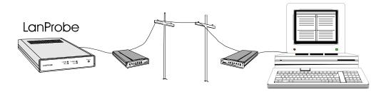
Figure 3-16: LanProbe Modem Connection
